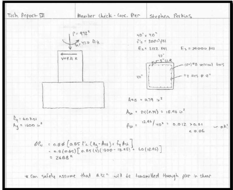
Figure 33: Design check of concrete pier
