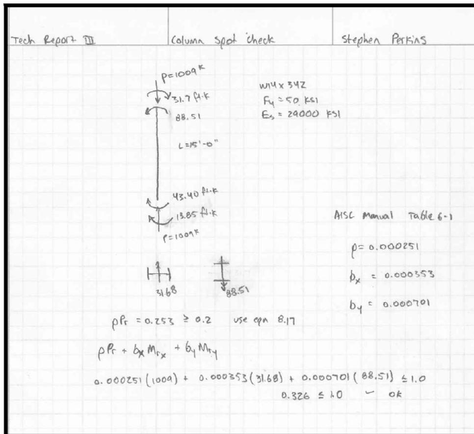
Figure 31: Column design check
