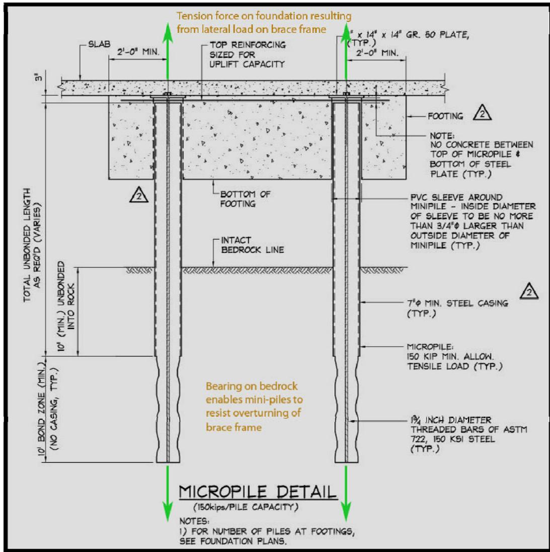
Figure 5: Mini piles are attached to the footing to resist tension forces.
