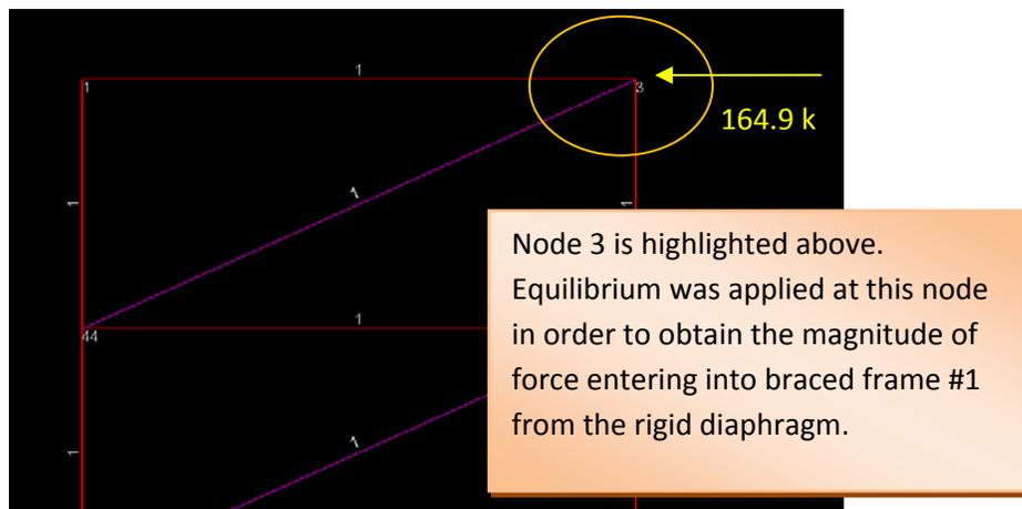
Figure 17: Equilibrium calculation for braced frames on tenth story.
