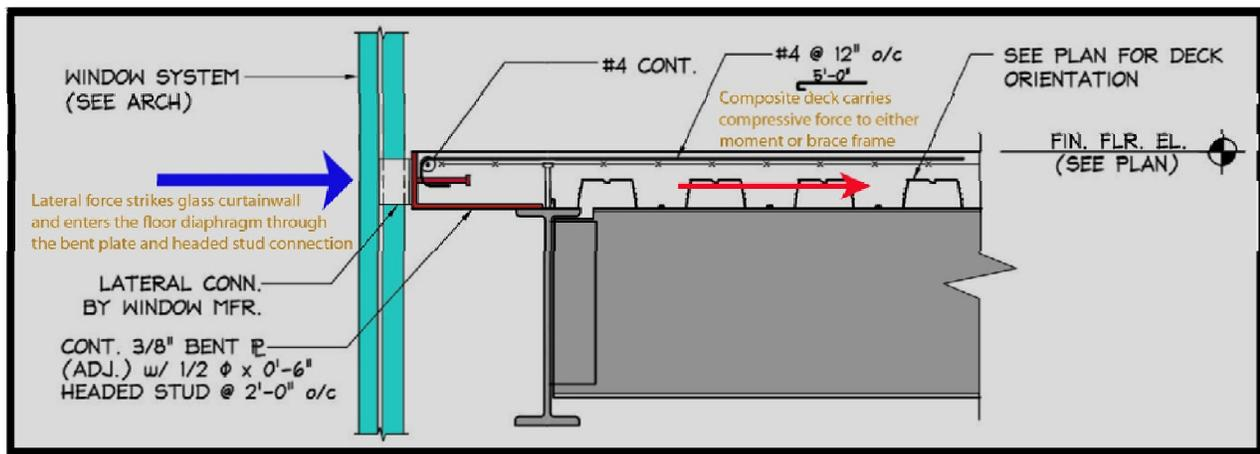
Figure 3: Lateral force enters the diaphragm from the façade and is carried to the braced and moment frames.
