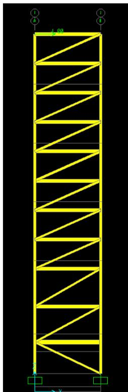
Figure 11: Braced Frame modeled in SAP2000.
