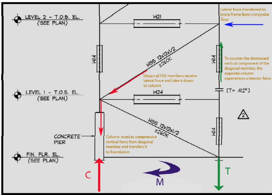
Figure 4: The above diagram shows how the lateral force is delivered into the foundation of the building through the diagonal braces of the frame.
