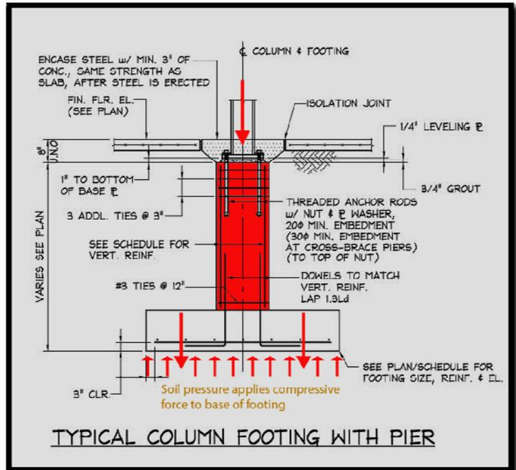
Figure 13: Connection at face of pier appears more fixed than pinned.
