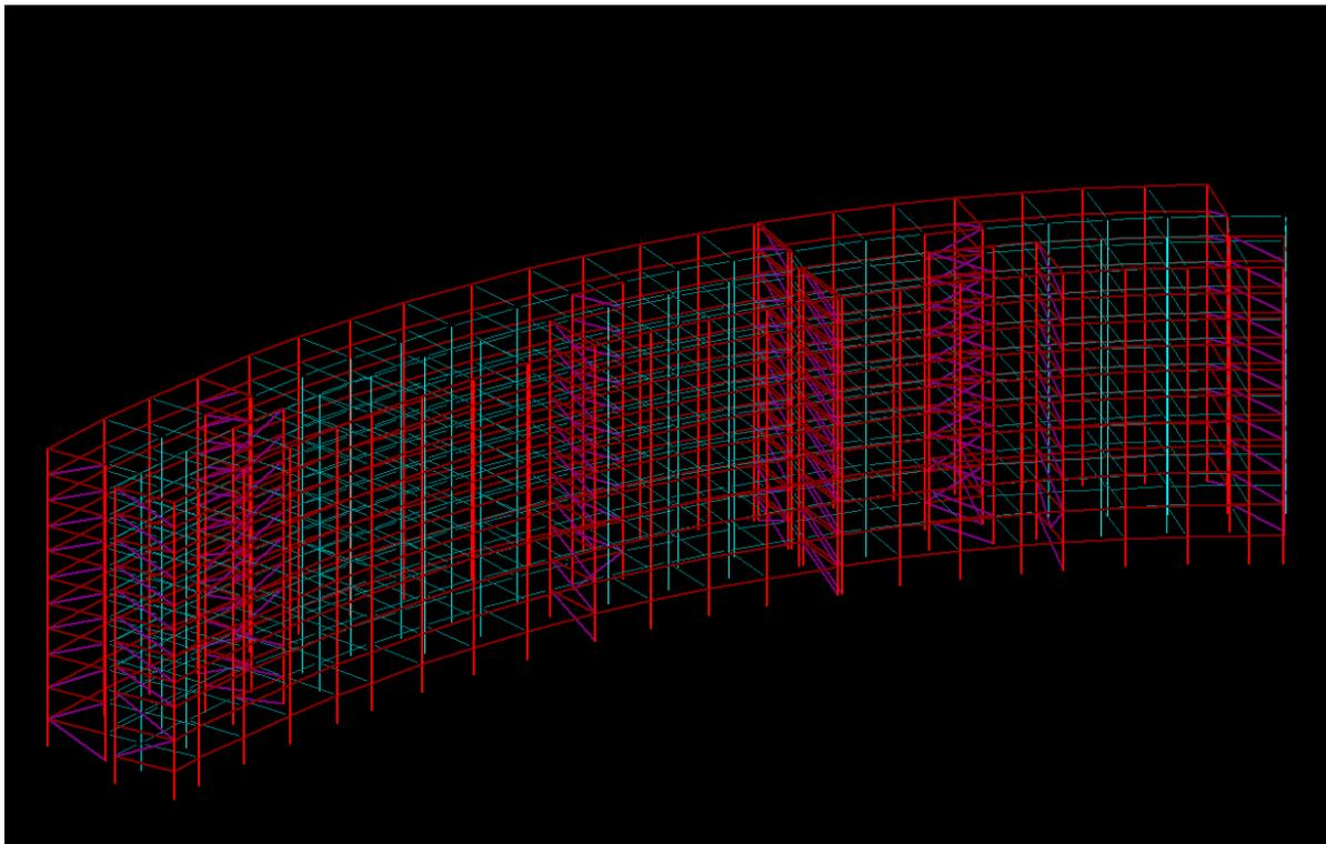
Figure 16: New Hospital modeled in RAM Structural System. Note the expansion joint near the middle.
