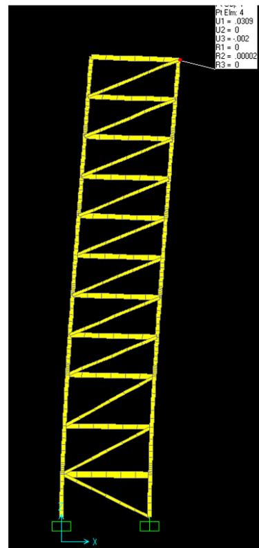
Figure 12: Displaced braced frame under 1 kip load.
