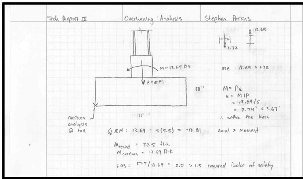
Figure 27: Overturning check
