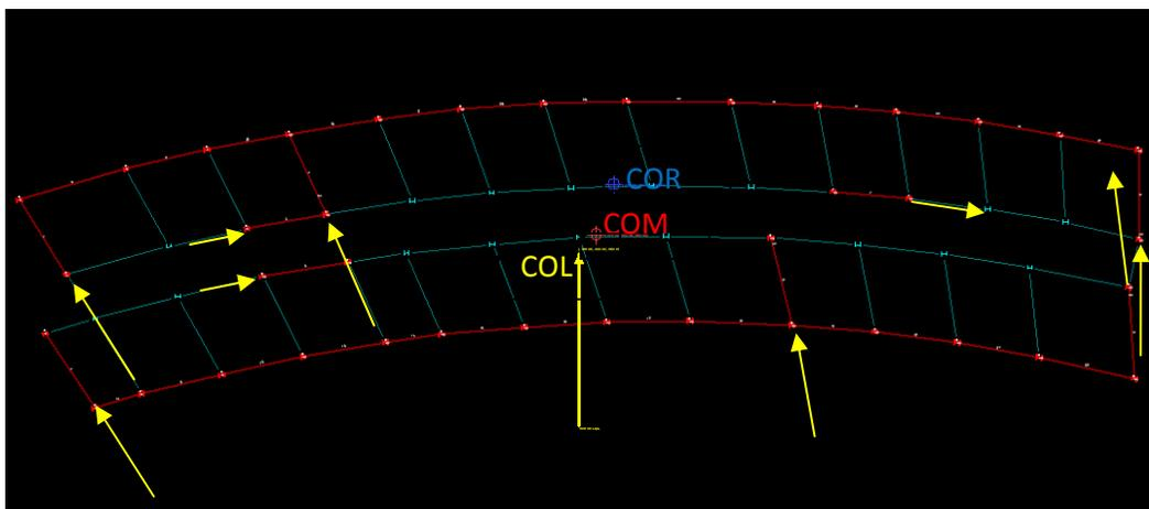
Figure 18: 1000 kip force applied at the center of pressure. Forces are then distributed based upon relative stiffness but remain in plane with the braced frame.
