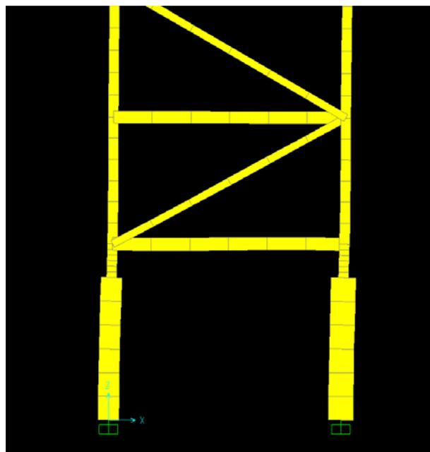
Figure 14: Close up view of concrete piers transmitting shear from the column and into the footing.
