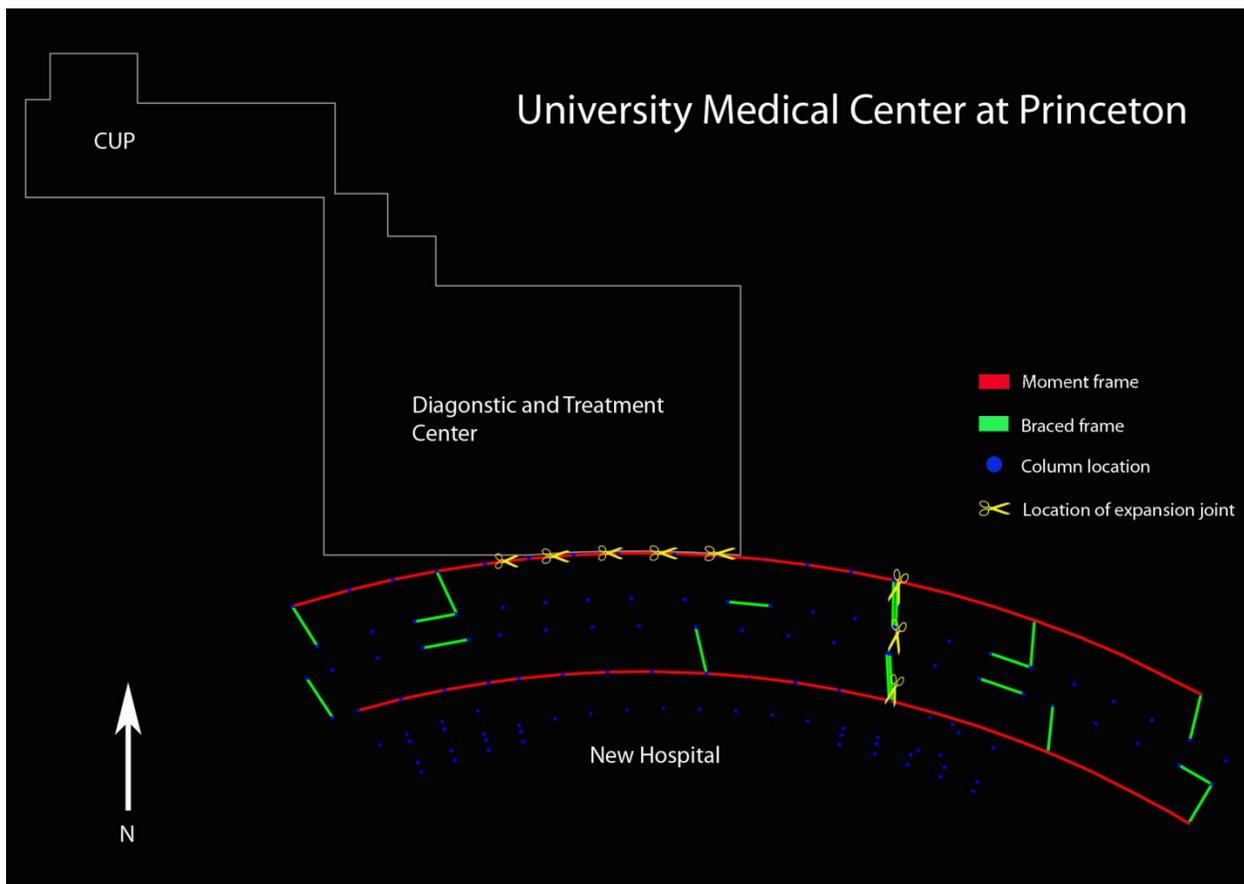
Figure 2: Overall schematic of lateral force resisting elements
